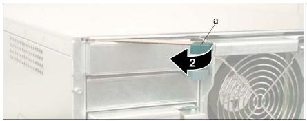
Figure 46: Disengaging the dummy module
